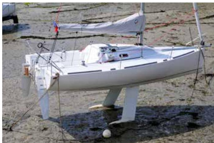
**The Yaka 650, an example of a neat twin-keel French cruiser developed from a Mini Transat 6.50 racer**
