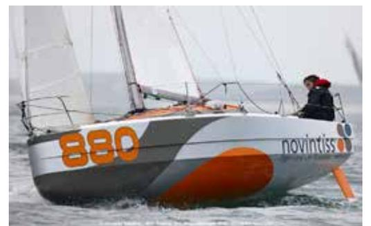
**Ofcet 6.50: one of these won 2015 Mini Transat 'Series' production class. The rounded bow and chines contribute to speed and stability**
