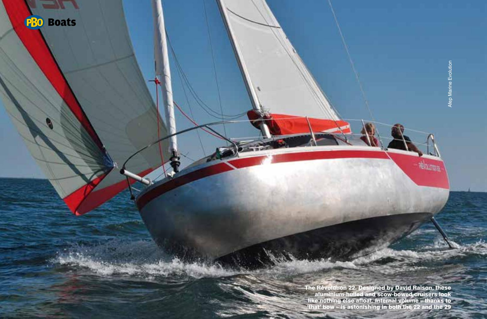
The Révolution 22. Designed by David Raison, these aluminium-hulled and scow-bowed cruisers look like nothing else afloat. Internal volume – thanks to ‘that’ bow – is astonishing in both the 22 and the 29
