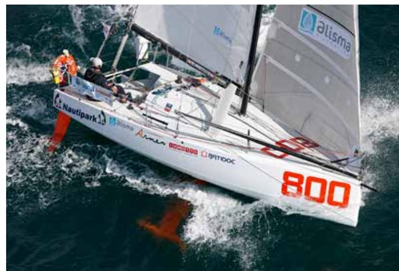
*Nautipark* (Frederic Denis) wins in the Proto class in 2015. Note the daggerboards, canting keel, chine, flat bottom and twin rudders
